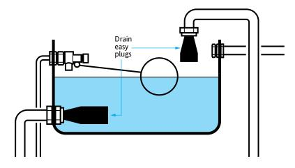
After releasing some inherent pressure in the system with the bleed key supplied, and building up a vacuum by allowing water to flow for about 1 minute, any single item such as a pump, valve or radiator may be removed without further loss of system water/inhibitor.
